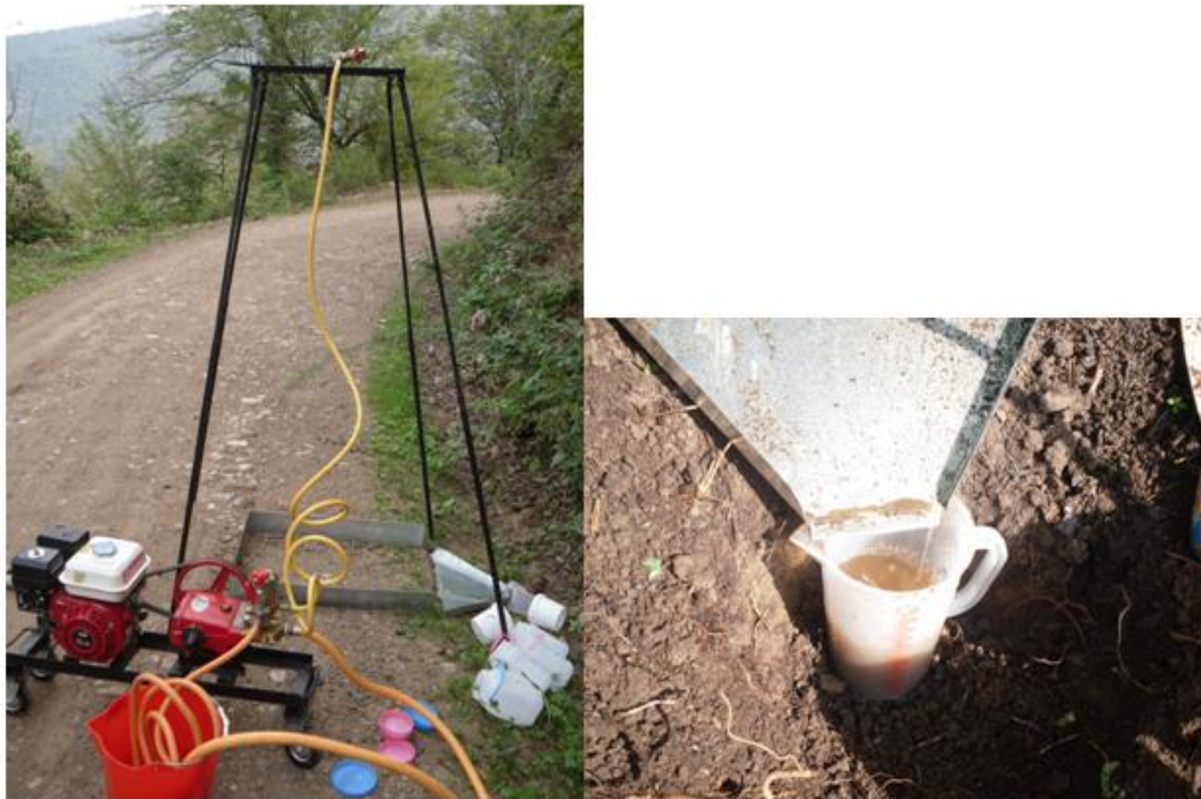
Figure 2. Rainfall simulator and runoff collection by the gauge.
